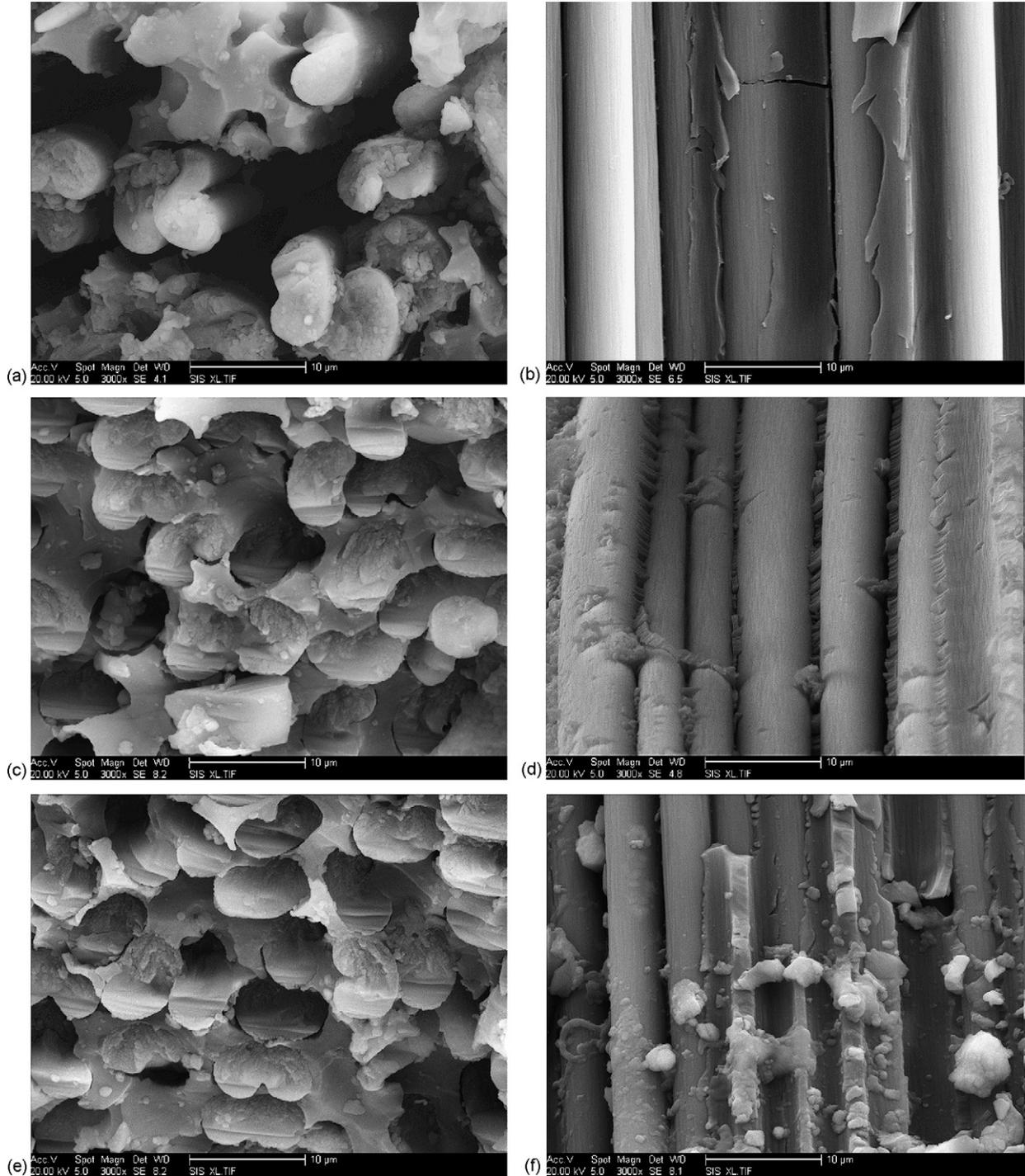
Fig. 6. SEM micrographs of fracture surface of composites: (a) cross-section of composites with untreated fibers; (b) side face of composites with untreated fibers; (c) cross-section of composites with immersion treated fibers; (d) side face of composites with immersion treated fibers; (e) cross-section of composites with irradiation treated fibers; (f) side face of composites with irradiation treated fibers.
