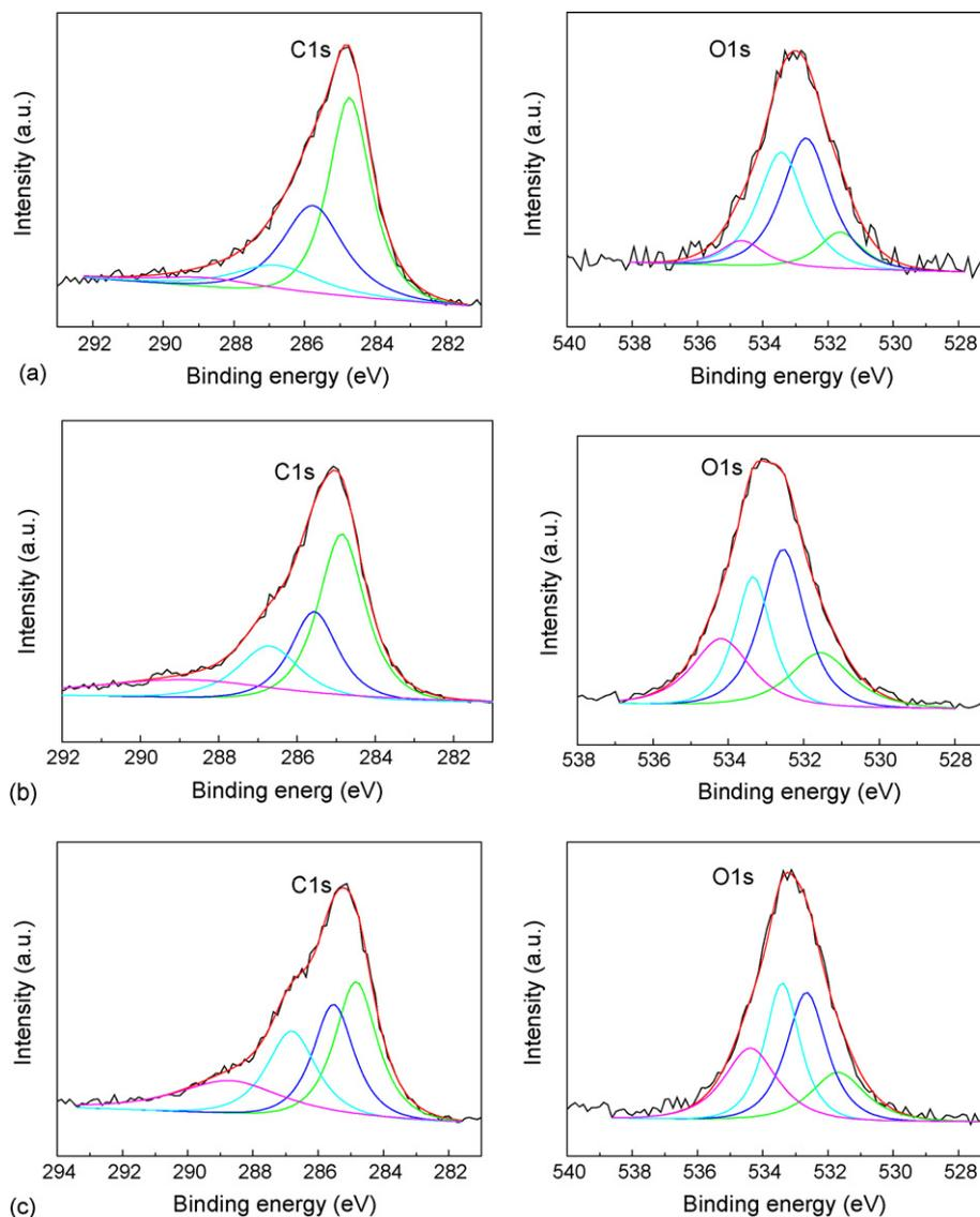
Fig. 3.  $C_{1s}$  and  $O_{1s}$  XPS spectra of carbon fibers untreated and treated: (a) untreated; (b) immersion treated; (c) irradiation treated.
