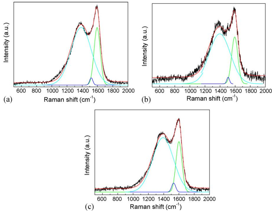
Fig. 4. Deconvolution of Raman spectra of untreated and treated carbon fibers: (a) untreated; (b) immersion treated; (c) irradiation treated.
