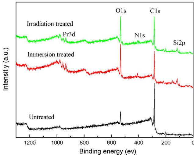
Fig. 2. Wide scan XPS spectra of untreated and treated carbon fibers.
