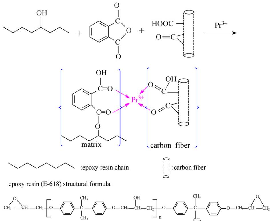
Fig. 7. Schematic diagram of coordination linkage between carbon fibers and matrix resin.
