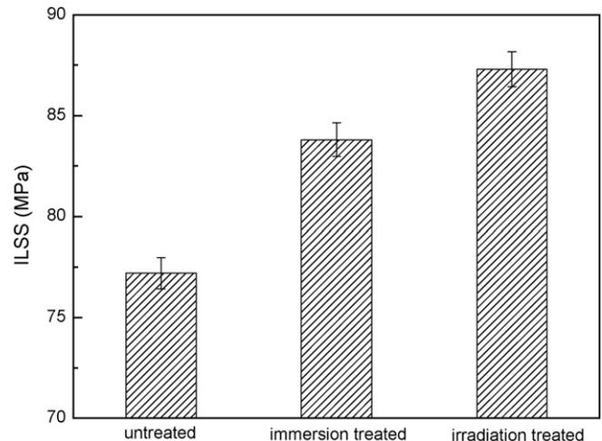
Fig. 5. Effect of treatment methods on ILSS of carbon fiber/epoxy composites.
