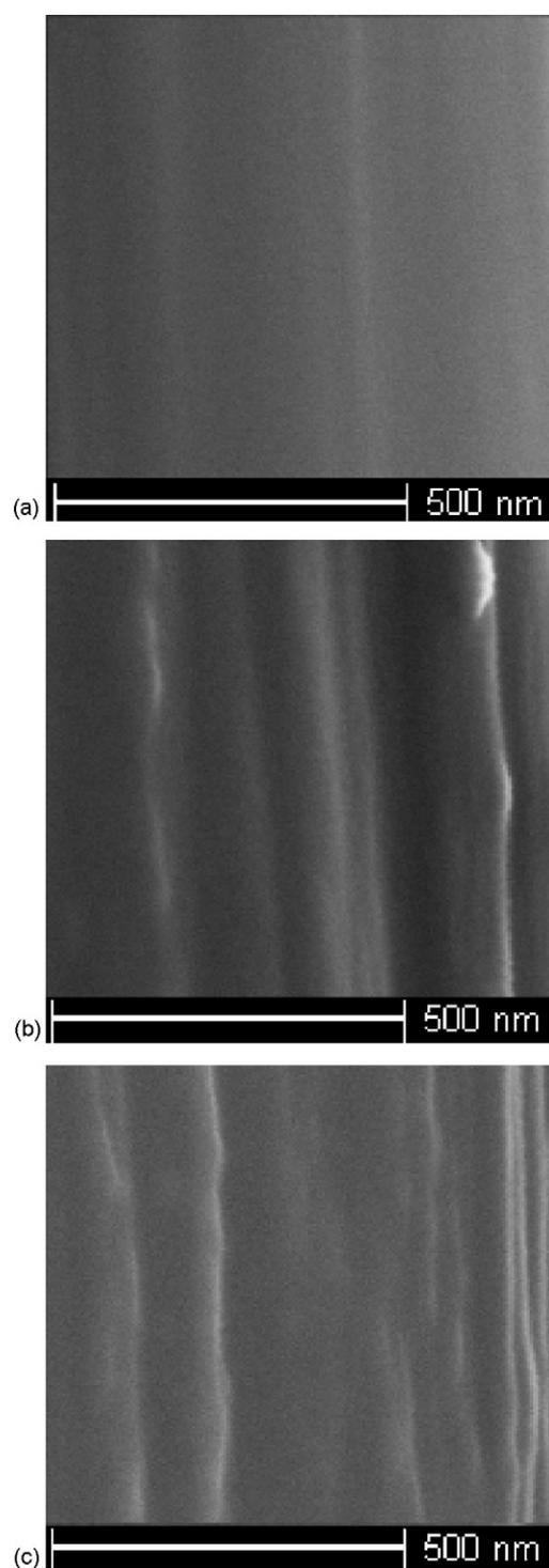
Fig. 1. Microscopic images of carbon fibers before and after treatment: (a) untreated; (b) immersion treated; (c) irradiation treated.
